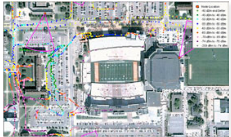
FIGURE 9 • Measuring signal strength outdoors to determine where to improve performance.
